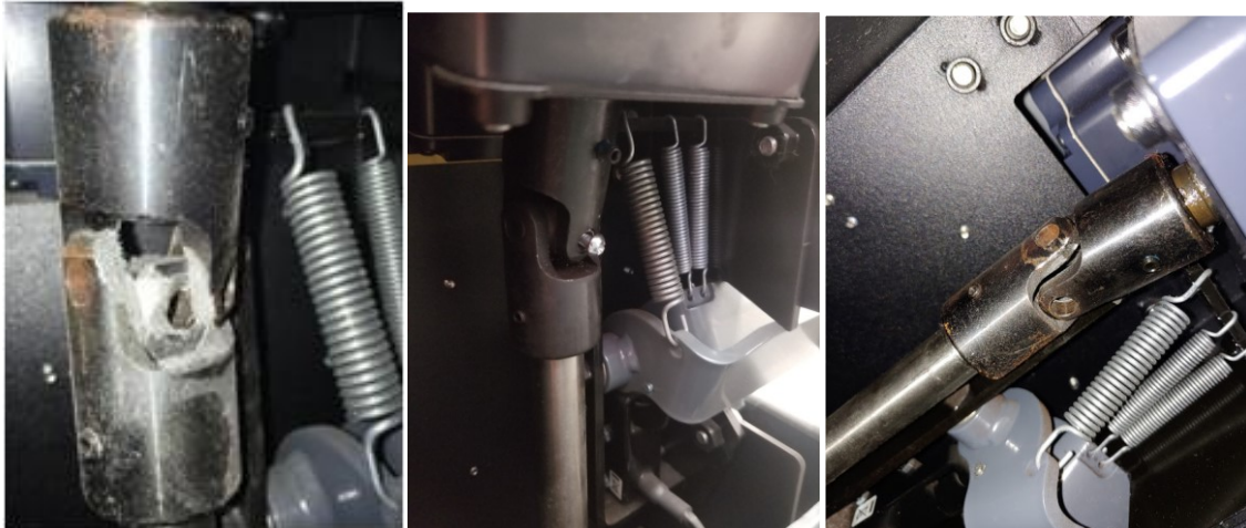
Example of a broken U-joint
