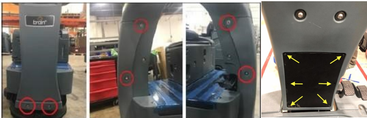
Removing both access
