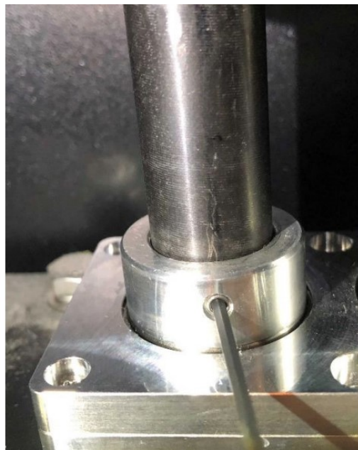
Loosen the collar (2 hex screws) and slide it down. Unplug the Steering Encoder connector.
